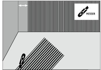
Cut the panels to the remaining width and mount them (screws or glue)
