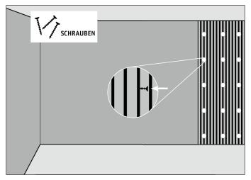
Attach the panels to the wall and screw or glue them in place.
