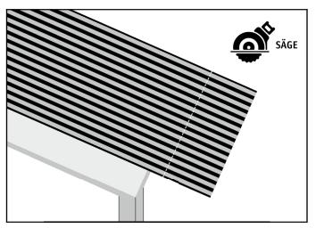
Cut the panels according to the height of the wall.
